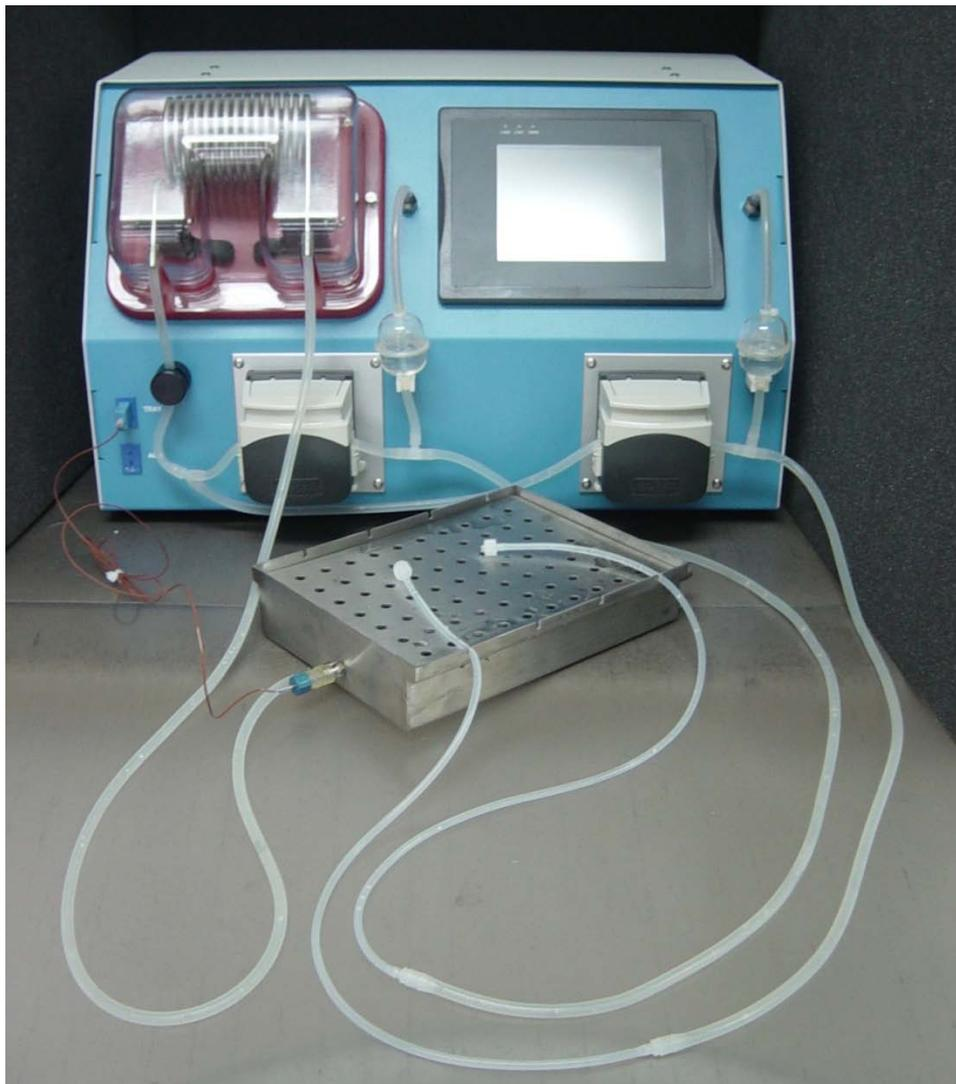
**Figure 10: Tubing Set and Tray Illustration**
